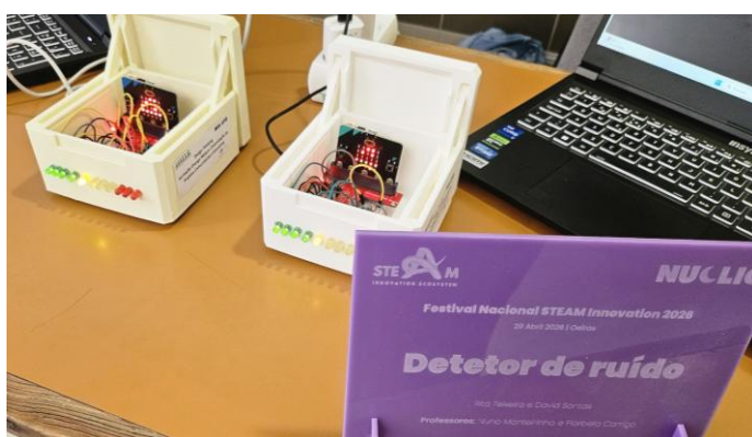
Figure 5: Final sound detector prototype developed by the students
