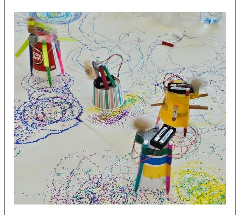
The way it works is very simple! The robot will move when it becomes unbalanced. This happens when the DC motor is connected to a part of its body that moves, causing an uneven distribution of weight. The circuit is very straightforward as well:
