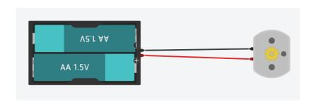
Since the DC motor is a bipolar electronic component, it will rotate regardless of how it is connected. However, it will rotate in the opposite direction if connected the other way.
