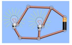
• Series-Parallel Circuit: Combine both series and parallel components by connecting some bulbs in series and others in parallel to explore how different configurations affect brightness and current flow. There are many configurations you can try out.
